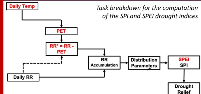
Task breakdown for the computation of the SPI and SPEI indices. The process consists in the computation of multi-day rainfall accumulation, distribution parameters, and drought indices.
