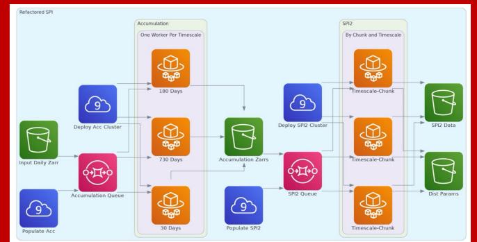
Task breakdown for the SPI source code adapted to the Amazon Web Services (AWS) cloud. The computational process is divided into three phases: file preparation (pre-processing), drought indices computation (accumulation periods, distribution parameters, SPI and SPEI computation), and output files finalization (size reduction, retiling, concatenation).
