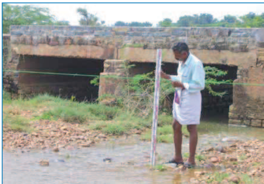
A stream gauge station for measuring outflow from the HU
