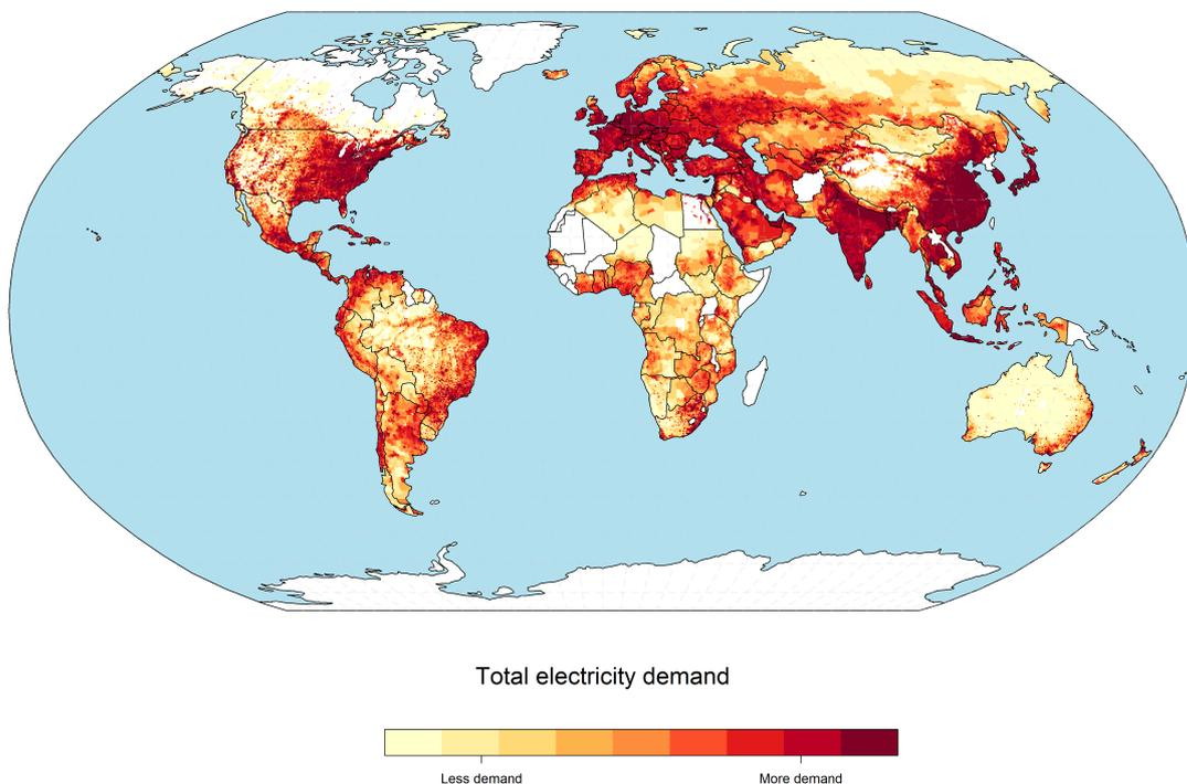
**Figure 11.** Map of total electricity demand by population, as the yearly national electricity consumption per capita (KWh) times population in 2015. Note that all non-domestic uses are included as well (Data sources: World Bank and CIESIN).
