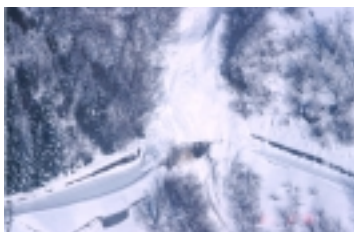
Figure 8. Example of a too short avalanche shed Bm/GL Switzerland (end of February 1999).
