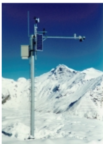
Figure 6 (left). IMIS network. Automatic snow and weather station at Simplon Pass, Valais Switzerland.
