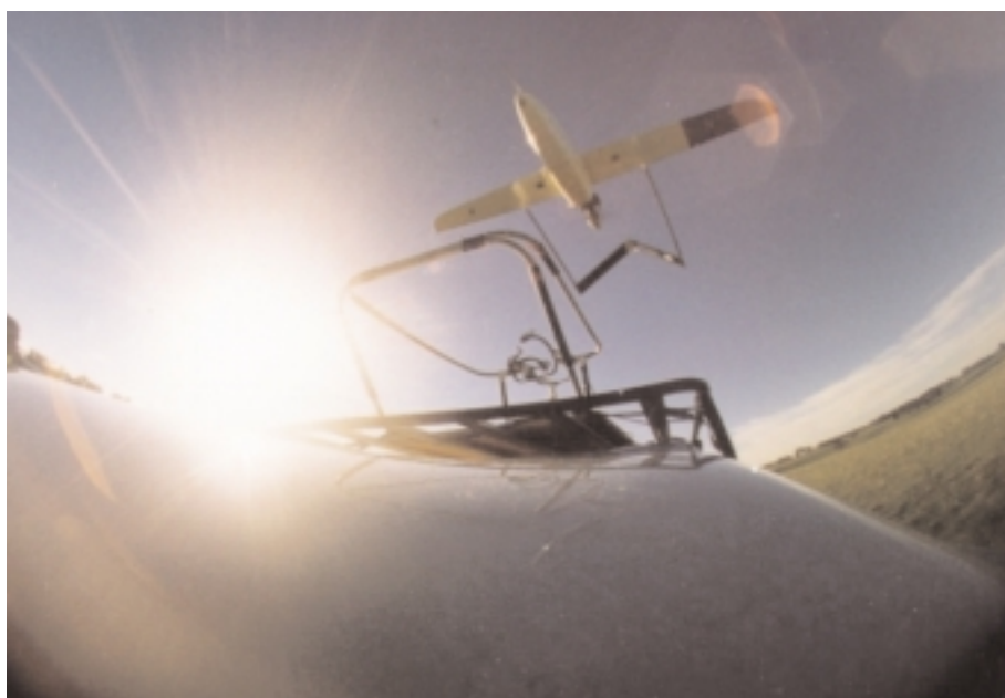
Figure 3. The Aerosonde Robotic Aircraft at launch from a car roof rack (K. McGuffie, personal communication 1998).
