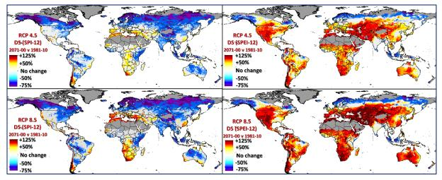
**Figure 2.** Drought severity (DS) according to the SPI-12 (left) and the SPEI-12 (right). All panels show the difference in percentage between 1981-2010 and 2071-2100 under the RCP4.5 (top) and the RCP8.5 (bottom) scenarios. Light grey zones represent areas in which less than two thirds of the simulations agree on the sign of change. Dark grey zones represent the cold and desert masked areas.
