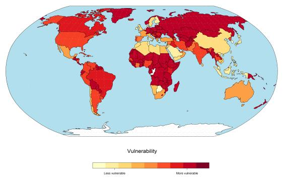
**Figure 12.** An example of a vulnerability map based on the ratio between power sources dependent and non-dependent from fresh waters. Power generators that do not need water for cooling or use seawaters have no vulnerability to droughts.
