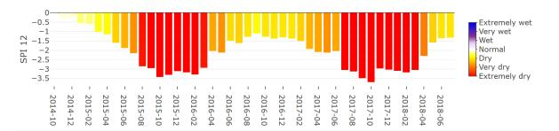
**Figure18.** Time-series of SPI with a cumulative period of 12 months (SPI-12) reaching extremely low values for many months, indicating a prolonged and severe hydrological drought.
